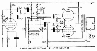
FIG. 7/16.—PP Amplifier with NFB applied over penultimate stage, with less reduction of gain than if fed into cathode of VI.
