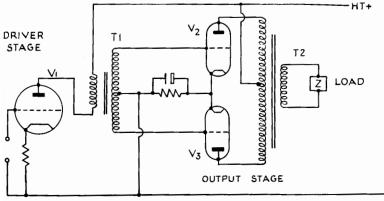
FIG. 6/2. Push-pull output stage.
