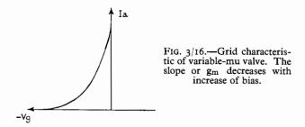
Reference to Fig. 3/16 shows the grid characteristic of a variable-mu valve. Comparison with the grid characteristics shown in Fig. 2/6 shows that the essential differences are that the point of cut-off is much more remote and that the characteristic is not truly straight over
