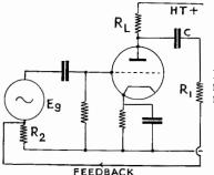
FIG. 7/7.—Amplifier with a fraction of the output *voltage* fed back in anti-phase to the input.
