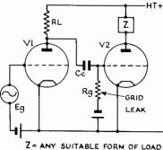
FIG. 3/5.—INTERSTAGE Resistance Capacity Coupling.
