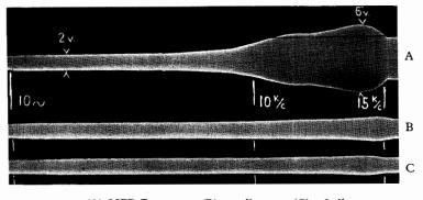
(A) NFB Zero (B) 14 db (C) 26 db FIG. 7/I.—Oscillograms showing effect of NFB on tetrode response.
