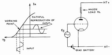
FIG. 3/4.-Grid Bias, to avoid grid current.
