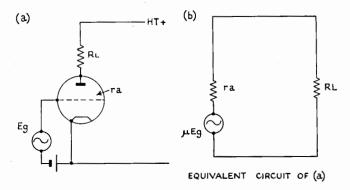
FIG. 4/2.—The valve as a generator.
