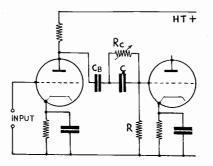
there is a cut of 3 db at 200 c/s or 1 db 400 c/s. However, as the value of  $R_c$  is reduced C is progressively shorted out, reducing the bass cut to zero at  $R_c$ =zero.
