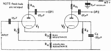
FIG. 9/6.—Cathode-coupled phase splitter.
