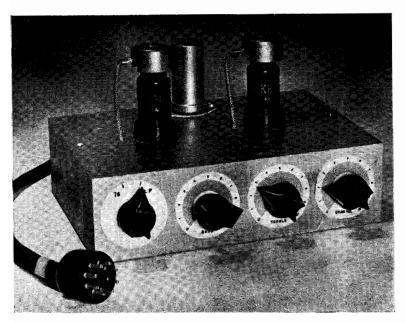
FIG. 17/12.—Pre-amplifier. Chassis  $8\frac{1}{2}$  ins. by  $5\frac{3}{4}$  ins. by  $2\frac{1}{2}$  ins. 8 by 8  $\mu$ F condenser at rear. VI left, V2 right. Note plug to main amplifier.
