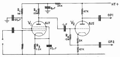
FIG. 9/8 .- A typical pre-amplifier and Concertina phase splitter stage.
