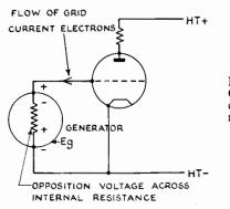
FIG. 3/2.—Effect of Grid Current. Opposition voltage developed across internal resistance of input voltage source.
