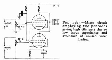
mixer circuit and a high stage gain achieved, due to the high anode resistance of the pentodes.
