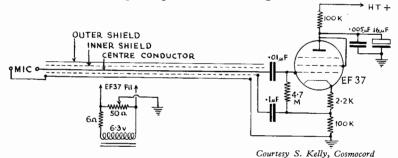
FIG. 13/9A.—Cathode follower input circuit. Input impedance 100M  $\Omega$ . Reduced heater volts are applied to the valve to reduce the effects of grid (gas) current flowing in the high value of grid leak.
