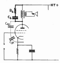
FIG. 5/8.—Feedback through inter-electrode capacities causing oscillation in output stage. R<sub>b</sub> and C<sub>b</sub> act as tone control by reducing higher frequencies, thus preventing oscillation.
