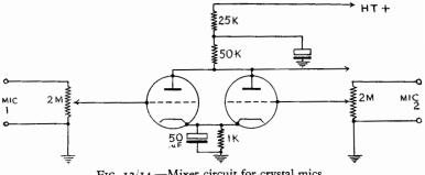
FIG. 13/14.—Mixer circuit for crystal mics. Cosmocord
