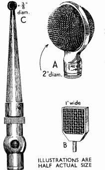
FIG. 13/7.—Crystal Microphones drawn to scale.
