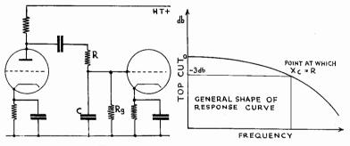
FIG. 10/4.—Basic treble cut circuit.
