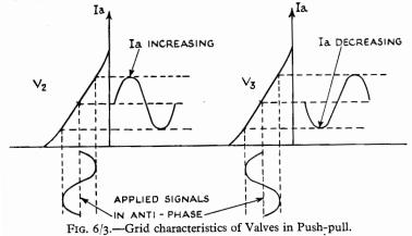
that the grids are operated in anti-phase on the straight part of their characteristic, with mid-point biassing known as the class A condition. The exciting voltage measured between the two grids will be twice that required for one valve, or parallel valves, but this presents little difficulty in practice, and the transformer T1 in Fig. 6/2 readily enables the grids to be fed in anti-phase. Other methods of obtaining the "phase split" are described in Chapter 9.
