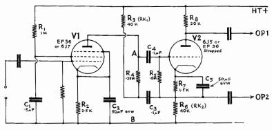
FIG. 9/9.—High gain phase splitter.
