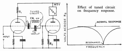
FIG. 10/1.—Circuit tuned to one frequency. Typical values for resonance at 9 Kc/s would be: CH=0.6H.  $C=.0005 \ \mu F$ .
