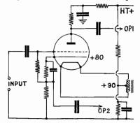
FIG. 9/2.—Modifications to Concertina Circuit. Arrangement to make heater of valve more positive than the cathode to avoid the effects of heater emission, and to avoid excessive voltage between heater and cathode. Separate heater winding is sometimes required.
