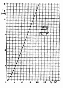
FIG. 2/4.—Anode Characteristic of Mullard DA90 Diode Valve.
