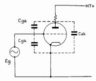
FIG. 3/10.—Inter-electrode capacities in a valve.
