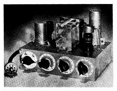
FIG. 17/13.—TRF Feeder and Pre-amp. Chassis 8½ ins. by 5<sup>3</sup>/<sub>4</sub> ins. by 2½ ins.
