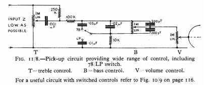
Since the valve following the control is usually the first valve of "flat" amplifier and has NFB applied to cathode, its input Z is very high and one need not worry about  $C_o$  existing from wiper of volume control to ground. NFB applied to cathode does not of course remove effect of any  $C_o$  due to screened leads, wiring, etc., but reduces  $C_o$  due to  $C_{gk}$  and  $C_{ga}$ .
