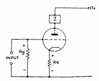
FIG. 3/13.—Cathode Biassing. Method of obtaining grid bias by resistance in cathode.
