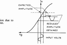
FIG. 3/3.—Distortion due to Grid Current.
