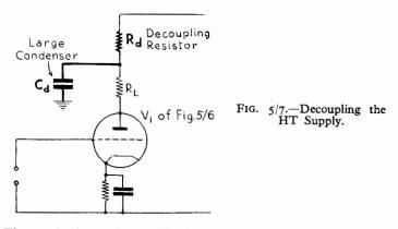
Figure 5/7 shows the modification that can be applied to  $V_1$  of Fig. 5/6. An additional resistance  $R_d$  is inserted between the HT supply and the load resistance  $R_L$  with a condenser  $C_d$  to the ground line from the junction of  $R_d$  and  $R_L$ .
