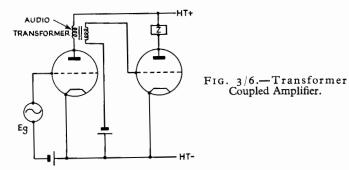
The primary of the transformer constitutes the anode load for V<sub>1</sub>, the secondary applies the voltage between the grid and cathode of V<sub>2</sub> and also supplies the DC path for the application of the bias voltage. This transformer can be of a step-up ratio primary to secondary, giving a
