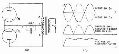
FIG. 14/6.-Basic bi-phase half wave Rectifier Circuit.
