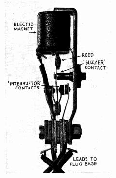
FIG. 14/14A. — Photograph showing working parts of vibrator.
