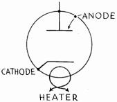
Typical directly heated valves consume 50 mA at 1.4 volts, 50 mA at 2 volts and a few legacies 1 amp at 4 volts. Typical indirectly heated types operate with 4 volts .65 to 1 amp, 6.3 volts .3 to .9 amps, 12 volts .15 amps, etc.
