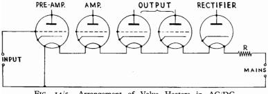
FIG. 14/5.—Arrangement of Valve Heaters in AC/DC Amplifier. Early valves at low potential end of chain.
