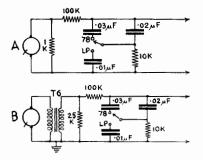
FIG. 11/4.—Bass lift circuit, with switch for 78 and LP matching, suitable for 400 ohms Connoisseur pick-up or other low impedance magnetic types. Increase value of R<sub>1</sub> for higher impedance coils or transformer input.
