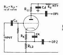
FIG. 9/1.—The single valve Concertina Phase Splitter.
