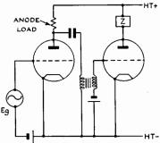
This is known as shunt or parallel feeding and enables a smaller transformer with lower self capacity but the same inductance to be used, but either method of using an interstage LF transformer is not regarded with much favour where the highest fidelity of reproduction is demanded. The transformer method of interstage coupling is frequently employed in radio circuits where the HF transformer will have an air core or dust iron core to avoid eddy current losses.
