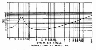
FIG. 4/3.—Typical loudspeaker impedance curve.
