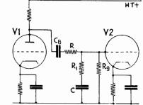
FIG. 10/6.—Typical bass lift circuit.
