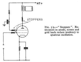
as the grid stopper and the capacity (R and  $C_{gk}$ , Fig. 5/10) form a low pass filter and attenuate the higher frequencies.  $R_1$  and  $C_{gk}$  behave as a potentiometer in which the reactance of  $C_{gk}$  becomes less with increase of frequency.
