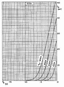
FIG. 2/6.—Grid Characteristic of Mullard EC52 Triode.
