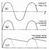
FIG. 14/2.—Voltage from Half Wave Rectifier.
