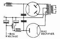
FIG. 14/12.—Power Circuit including a fixed GB supply.
