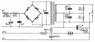
FIG. 14/17.—Complete vibrator pack. Metal rectification is employed for reasons of valve heater economy. Note RFC's + bypass condensers to eliminate RF ripple.
