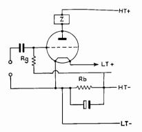
FIG. 3/15.—Back biassing, or HT- lead biassing.
