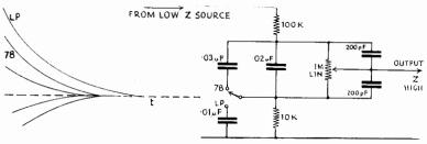
FIG. 11/6.—Variable bass control with 78/LP switching.
