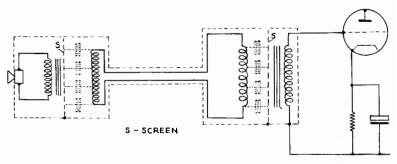
FIG. 13/8A.—Input circuit with stray capacities balanced to avoid hum. Suitable line impedance would be 600 ohms.
