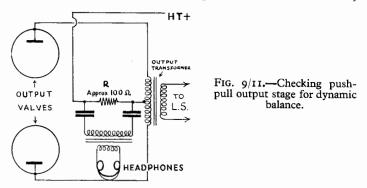
both, are a very necessary safety precaution when wearing headphones connected to the HT+ supply.
