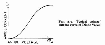
be seen that at low anode voltages the current increases but slowly. Then, as the anode is made more positive, the electron current grows rapidly, then less rapidly, and finally remains constant. Any further
