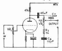
can be obtained. In general one rather neglects the treble boost as the falling off of the ear is not so rapid as in the bass. The simple circuit of Fig. 10/13 will afford a degree of bass compensation.
