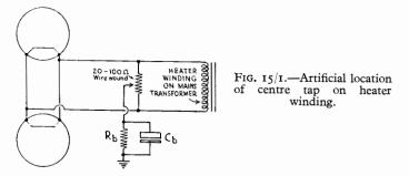
If the output stage is push-pull, unbalance of current in output transformer windings due to bad mis-match between the valves may be the cause of hum. Check anode currents with both grids earthed. If removal of earths on grids causes change in anode currents suspect grid-earth return paths. If removal of earth on grids increases hum
