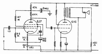
FIG. 8/7.—Comparable amplifier to that of Fig. 8/5, but arranged for tetrode output with variable voltage NFB overall.
