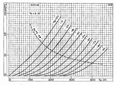
FIG. 2/7.-Anode Characteristic of Mullard ECC33.
