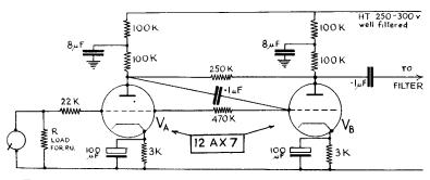
FIG. 11/9.—Pre-amplifier with low output impedance designed to feed into filter circuit of Fig. 11/8. Input circuit for magnetic pick-up.
