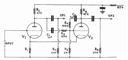
FIG. 9/7.—The Anode Follower, which is the modified version of the "Floating Paraphase" of Fig. 9/5.
