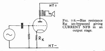
will increase and therefore the voltage developed across  $R_K$  will be greater. This will reduce the effective input volts still further, causing a decrease in anode current which tends to offset the original rise due to the reduced value of load  $R_L$ , *i.e.* the feedback is tending to make the value into a *constant current* generator.
