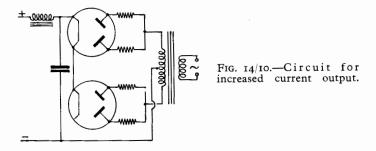
Mullard PZ30 and Mazda U801 which are rated to supply 200 mA and 300 mA respectively, these having separate diodes in the one envelope.
