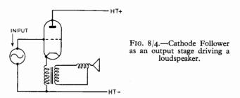
loudspeaker via the transformer is the optimum load quoted for the particular valve employed.
