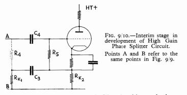
9/10 can be connected to HT+ as in Fig. 9/9 with exactly the same result in the AC sense, HT+ being at earthy potential.  $R_4$  shown dotted in Fig. 9/10 is a necessary addition to the circuit to provide HT feed for  $V_1$  and whilst the DC resistance is about 0.25M the impedance is, say, 1.6 megohms (0.2M + .5M in parallel × 10) because of the NFB (neglecting negligible reactances of  $C_3$  and  $C_5$ ).
