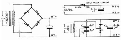
FIG. 14/9.—Typical Metal Rectifier Circuits.
