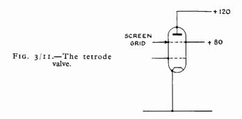
This greatly reduced the anode to grid capacity but did not completely eliminate it. Examination of the grid characteristics of typical screen grid or tetrode valves shows them to be not dissimilar to those of an ordinary triode.
