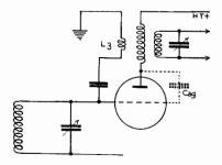
FIG. 17/14.—Stabilising RF amplifier by introducing out of phase feedback to cancel effects of inter-electrode capacity and stray couplings. GARNER AMPLIFIER
