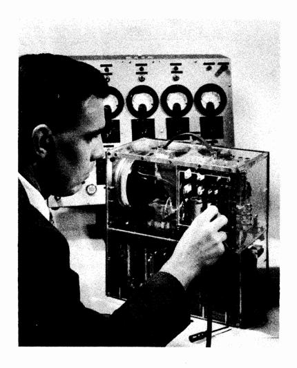
An experimental portable TV Receiver using only one tube the Picture Tube. This receiver is representative of the type of equipment the serviceman may one day be called on to service and maintain. A knowledge of transistor operation is essential to the proper maintenance of such equipment.
