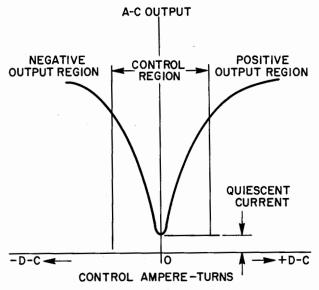
Fig. 37. Transfer characteristic curve.
