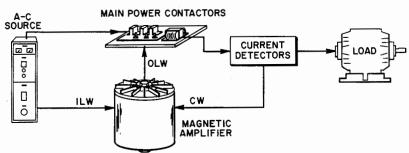
Fig. 81. Overload trip device.
