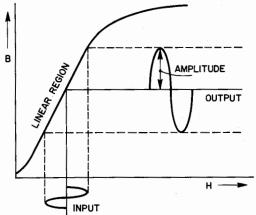
Fig. 35. Amplification in a simple saturable reactor.
