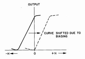
Fig. 55. Result of bias winding.
