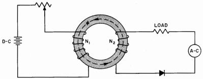
Fig. 44. Transformer action of two windings.
