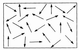
showing the direction of the domain. When an external force is capable of causing these tiny magnets to align or orient themselves so that they are pointing in the same direction, the magnetic material is said to be magnetized (Fig. 7A).
