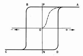
Fig. 101. Square hysteresis loop for magnetic cores.
