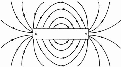
Fig. 10. Magnetic field around bar magnet.
