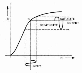
Fig. 33. Distorted output waveform.
