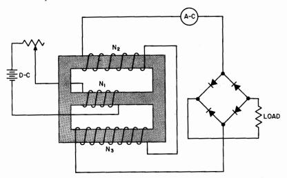
Fig. 48. Magnetic amplifier with rectifier bridge in output.
