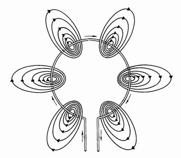
Fig. 15. Magnetic field around current-carrying loop.
