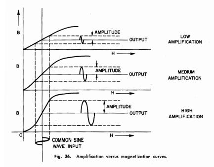
Fig. 36 shows the effects on amplification of operating with varying slopes of different core material. The core material having the greatest slope is capable of high amplification, while the core material with least slope has a lower amplification.
