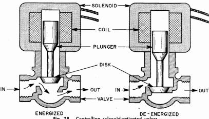
Fig. 78. Controlling solenoid-activated valves.
