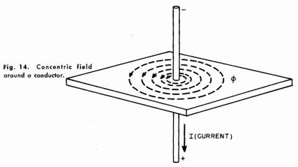
To determine the direction of a magnetic field around a conductor, grasp the conductor with the left hand, pointing the thumb in the direction of current flow. The fingers will then point in the direction of the magnetic field.
