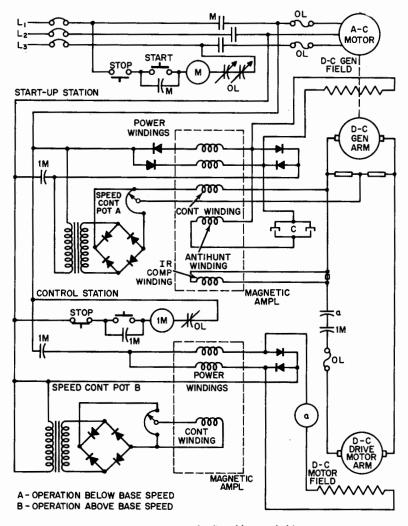
Fig. 89. Diagram of adjustable speed drive.
