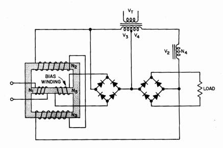
Fig. 54. Compensated magnetic amplifier with bias.
