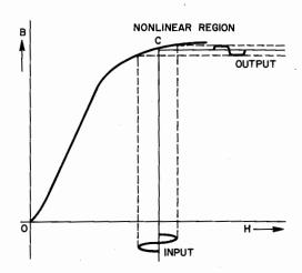
Fig. 34. Highly distorted output waveform.
