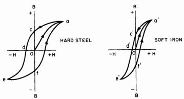
Fig. 22. Hysteresis loops for soft iron and steel.
