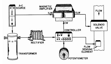
Fig. 79. Control of solenoid actuator valves.
