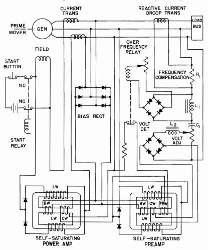
Fig. 91. Automatic line voltage regulator.
