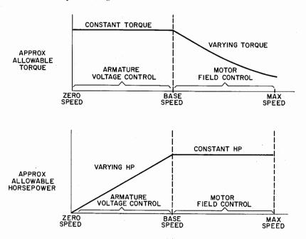
Fig. 88. Motor torque and horsepower curves.
