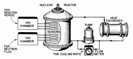
Fig. 95. Malfunctions are detected by sensors.
