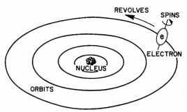
Fig. 5. Electron revolving around nucleus and spinning on its axis.
