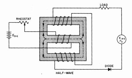
Fig. 38. Self-saturating magnetic amplifier.
