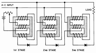
Fig. 50. Cascaded magnetic amplifiers.
