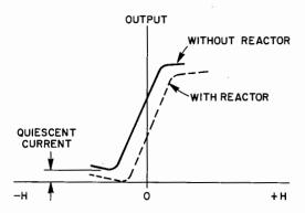
Fig. 52. Effect of adding compensating reactor.
