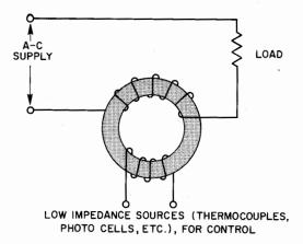
Fig. 73. Load windings may be matched to laad impedances.
