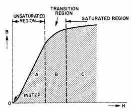
Fig. 21. Regions of the magnetization curve.
