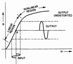
Fig. 32. Output wave when operating in linear region.
