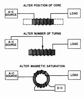
Fig. 69. Variable reactance methods.
