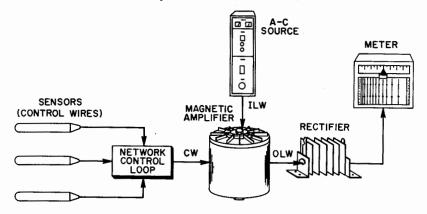
Fig. 86. D-c metering of large power lines.
