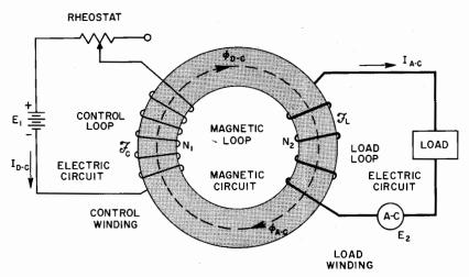
Fig. 30. Simple saturable reactor.
