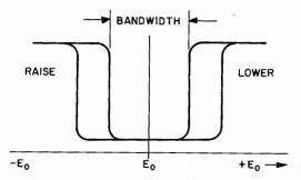
Fig. 93. Bistable output of a magnetic amplifier.
