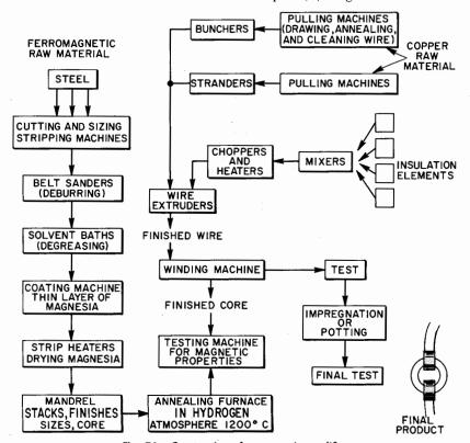
Fig. 74. Construction of a magnetic amplifier.
