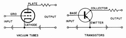
Fig. 65. Adjustable current devices.
