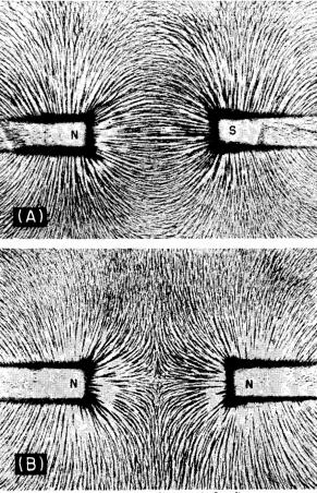
Fig. 12. Pattern of magnetic flux lines.
