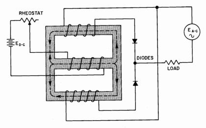
Fig. 39. Full-wave self-saturating magnetic amplifier.
