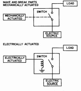
Fig. 70A. Make and break parts mechanically actuated.
