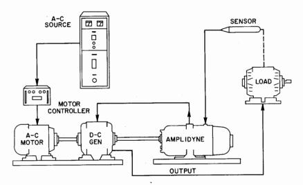
Fig. 66. Adjustable voltage system.
