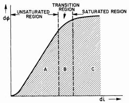
Fig. 25. Magnetization effects on inductance.
