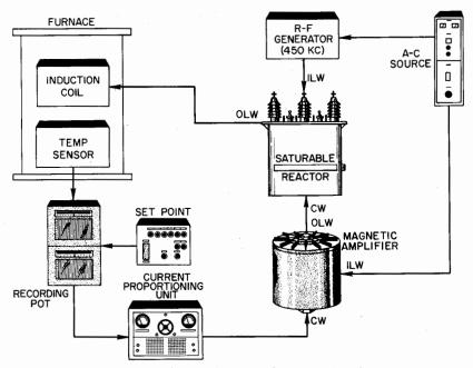
Fig. 83. Control system for semiconductor crystal production.
