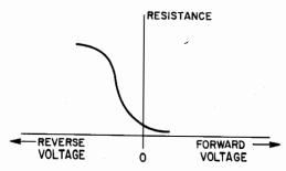
Fig. 40. Diode resistance versus applied voltage.
