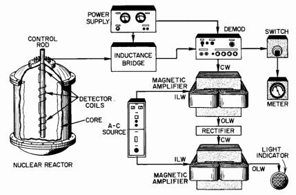
Fig. 96. Indicating system for position of control rod.
