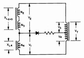
Fig. 53. Schematic diagram of a compensated magnetic amplifier.
