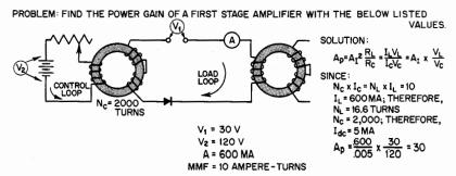
Fig. 61. Power gain is the ratio of the output to the control circuit power.
