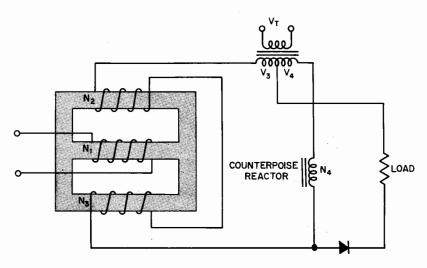
Fig. 51. Compensated magnetic amplifier.
