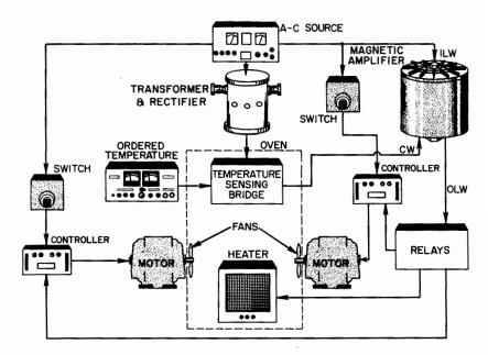
Fig. 84. Temperature control system.
