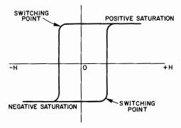
Fig. 64. Bistable operation of magnetic amplifier.
