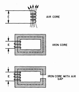
Fig. 26. Three basic types of simple magnetic circuits.
