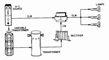
Fig. 80. Light dimming control system.
