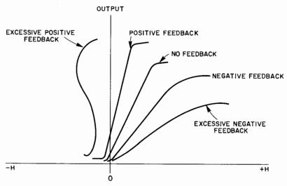
Fig. 63. Effect of feedback on transfer characteristic.
