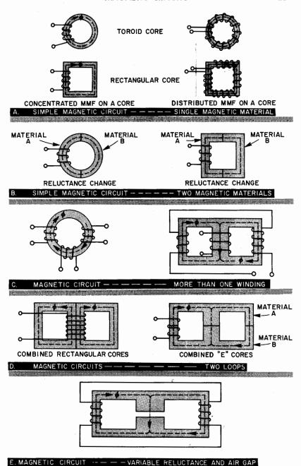
Fig. 28. Types of magnetic circuits.
