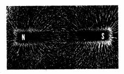
field is often referred to as lines of flux, or simply flux. They are often designated by the symbol " $\phi$ ". The unit of flux is one line and is called the maxwell. The flux per unit area, or the number of maxwells, is known as the flux density and is designated "B". The unit of flux density, or one maxwell per square centimeter, is called gauss. Therefore, by definition:
