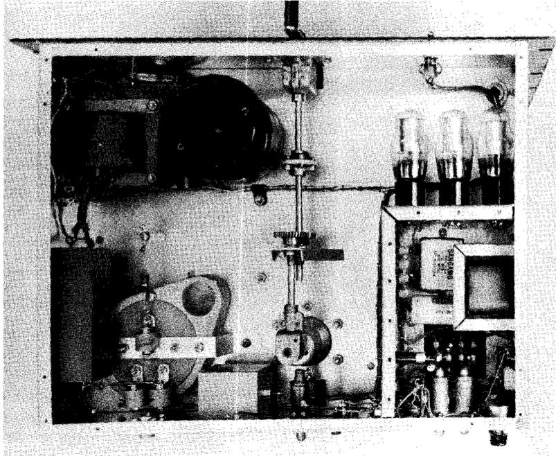
shield is  $9\frac{3}{8}$ " high. This shield is made of one piece of aluminum, bent into a U-shape, having  $\frac{1}{2}$ -inch flanges on all sides. The open side of the "U" is bolted to the front panel as shown in the photographs. Elastic stop-nuts are affixed to the shield every  $1\frac{1}{2}$ " along the flange, or it may be drilled and tapped for 6-32 machine screws. A shield of this type can be homemade, or it may be fabricated in any large sheet metal shop for a small sum.
