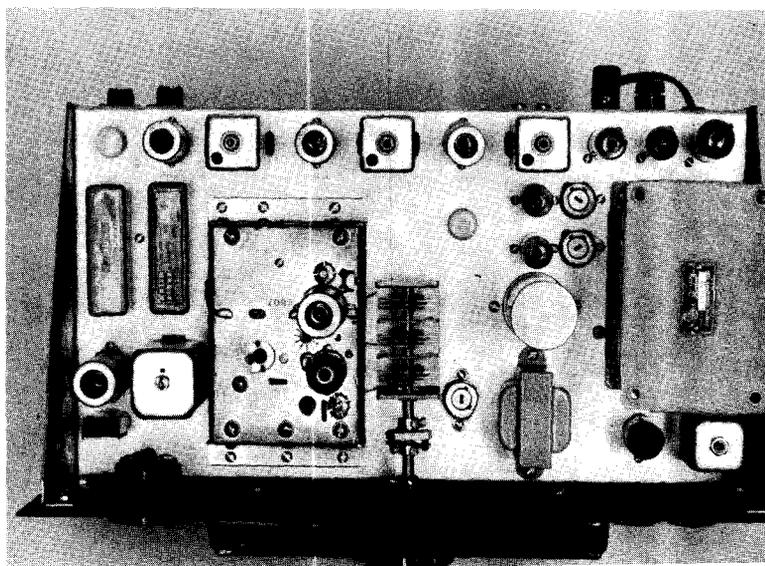
age regulator tube, and the 12AU7 S-meter tube. In front of the last i-f transformer can be the two 6AL5 tubes and potentiometers  $R_6$  and  $R_7$ .
