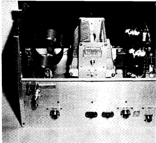
supporting the sockets. The complete amplifier is enclosed in a shield made of aluminum. Holes are drilled above the 803 tubes in the top sheet (figure 25) and in the rear plate to permit circulation of air about the tubes.
