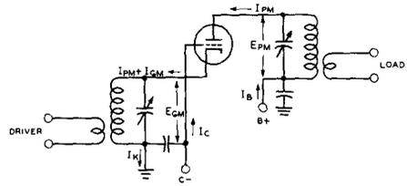
$$\text{POWER OUTPUT TO LOAD} = \frac{(E_{GM} + E_{PM}) I_{PM}}{2} \text{ OR } \frac{E_{PM} I_{PM}}{2} + \frac{E_{GM} I_{PM}}{2}$$
