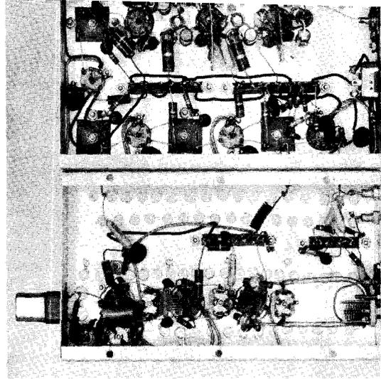
vides the proper mixing voltage for this stage. Three stages of 6BA6 amplifiers at 4.5 Mc. comprise the i-f section of the receiver. A-v-c is applied to each stage. A 6T8 multi-purpose tube ( $V_7$ ) is employed as diode detector, a-v-c rectifier, noise limiter, and first audio stage.
