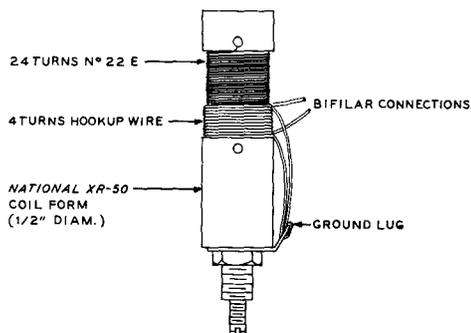
NOTE: TWO PARALLEL PIECES OF HOOKUP WIRE ARE WOUND SIMULTANEOUSLY OVER PRIMARY WINDING TO MAKE BIFILAR SECONDARY. BOTTOM END OF ONE WINDING AND TOP END OF OPPOSITE WINDING ARE GROUNDED TO MOUNTING LUG ON COIL FORM.
