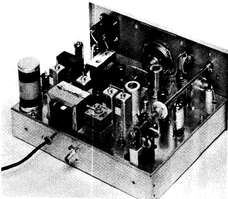
section of the unit occupies the center section of the chassis with the power supply directly behind it. To the right is the transmitter section with the variable frequency oscillator at the rear. Panel control of the oscillator is accomplished by an extension shaft and a flexible coupling. At the left of the chassis is the audio system.
