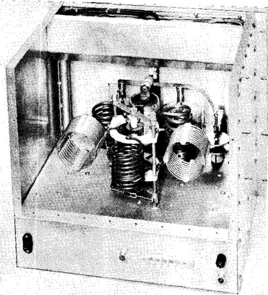
position high voltage ceramic rotary switch. Each coil is adjusted for optimum circuit Q, resulting in no tank circuit compromise in efficiency at the higher frequencies. A close-up of the tank circuit is shown in the introductory photograph at the chapter head, and complete coil data is given in figure 39. The plate blocking capacitor is made of two .001  $\mu$ fd., 5 KV ceramic capacitors connected in series.
