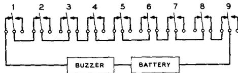
NOTE: ALL BUTTONS HAVE ONE NORMALLY OPEN CONTACT AND ONE NORMALLY CLOSED CONTACT.
