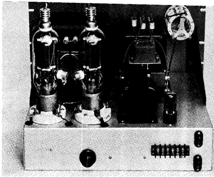
The modulator chassis includes a small low impedance bias supply capable of delivering approximately —75 volts under the changing load conditions imposed by the varying grid circuit impedance of the class B modulator.
