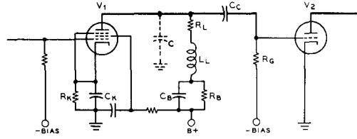
MID-FREQUENCY GAIN =  $G_{M V1} R_L$
