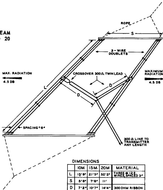
to one-quarter wave spacing may be used on the fundamental for the one-section types and also the two-section center-fed, but it is not desirable to use more than 0.15 wavelength spacing for the other types.
