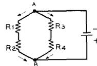
In this type of circuit the resistors are arranged in series groups, and these seriesed groups are then placed in parallel.
