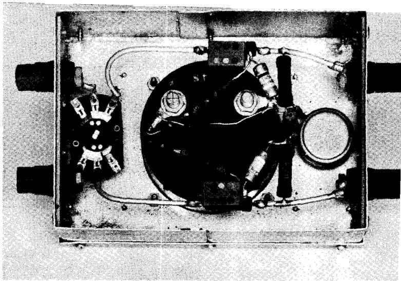
broken by two 250 ohm composition resistors and switch  $S_1$ . The line segments are made of short pieces of #10 copper wire, running between the various components. Spacing between the wires is held close to three inches to approximate a 500-600 ohm line.
