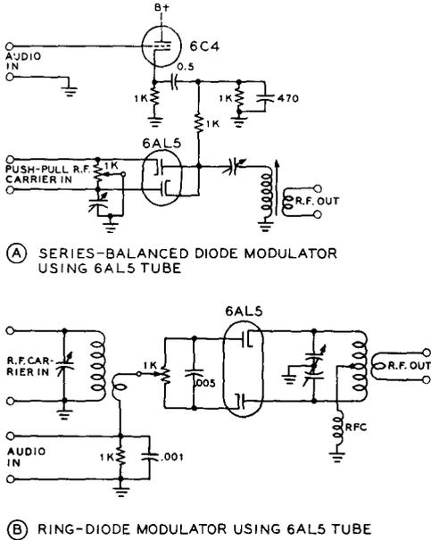
(A) SERIES-BALANCED DIODE MODULATOR USING 6AL5 TUBE
