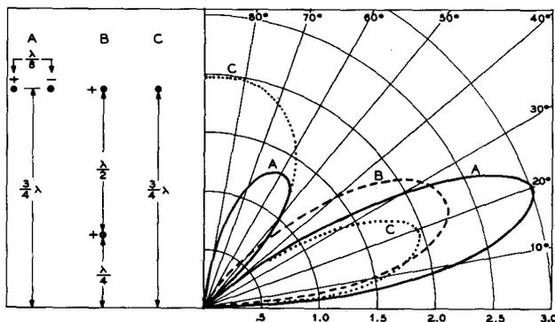
angle radiation at the expense of the useless high-angle radiation with these simple arrays as contrasted to the dipole is quite marked.
