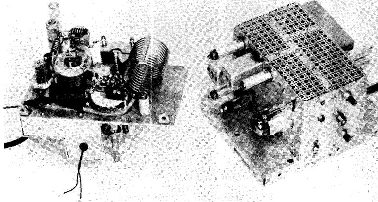
clearly visible in figure 32. The clearance space provided by the "step" is occupied by the "SSB-standby-CW" switch  $S_1$  which is mounted to the panel in close proximity to the grid circuit components of the amplifier stage. The important leads to the control switch pass out of the grid compartment through ceramic feed through capacitors mounted on the wall of the "step" shield. The coaxial r-f output lead and the grid bias lead also pass through this shield and may be seen in figure 32.
