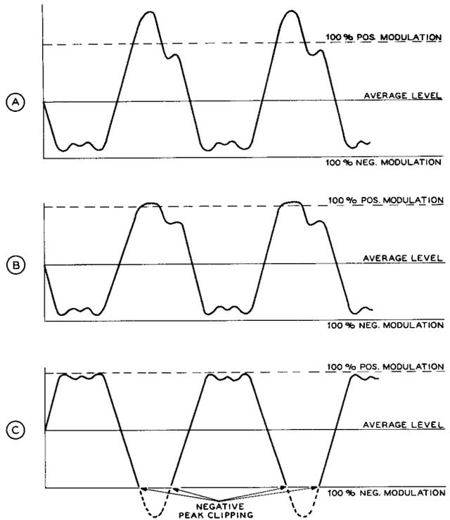
negative peaks of modulation. This aspect of the problem has been discussed in more detail in the section on *Speech Waveform Dissymmetry* earlier in this chapter. The effect of feeding the proper speech polarity from the speech amplifier is shown in figure 14.
