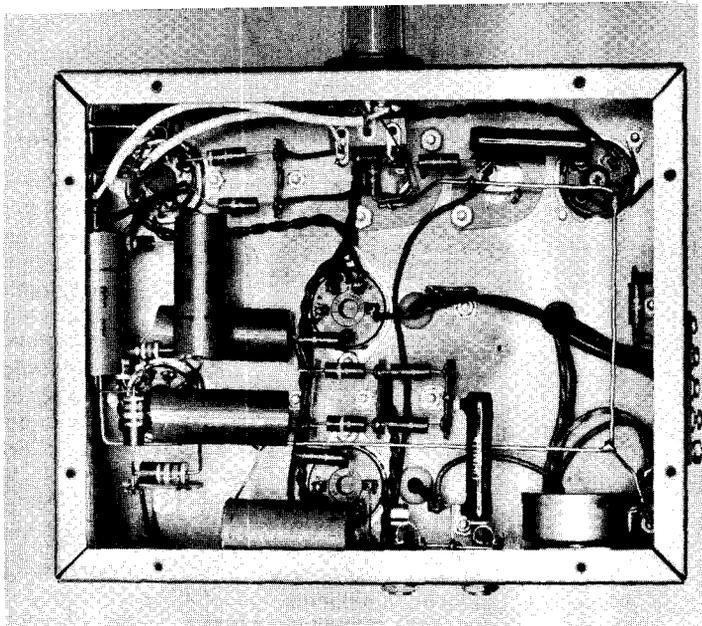
driver stage for the high level output amplifier. A plate potential of 430 volts is applied to this stage to insure ample grid drive to the output stage. Large value coupling capacitors are used between all stages to prevent signal degeneration at the lower audio frequencies. Two 807 beam-power tubes are employed in the final amplifier stage. Cathode bias is applied to these tubes, and the current of the tubes may be equalized by potentiometer  $R_2$  in the bias circuit.
