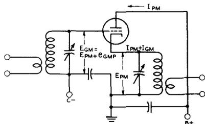
POWER OUTPUT TO LOAD =  $\frac{E_{PM} (I_{PM} + I_{GM})}{2}$
