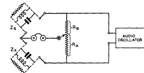
$$Z_x = \frac{R_A}{R_B} Z_s \qquad X_x = \frac{R_A}{R_B} X_s \qquad R_x = \frac{R_A}{R_B} R_s$$
